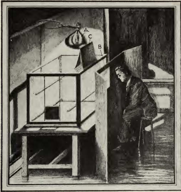
Figure 1. Dark observation room. A. Nickel-plated reflector with 150-watt bulb. B. Transparent mirror. C. Cardboard shade to prevent reflection on transparent mirror.
